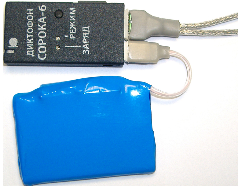
Fig. 9. Example of the voice recorder "SOROKA(Forty) - 06" operation with an external accumulator and external stereo microphones.
